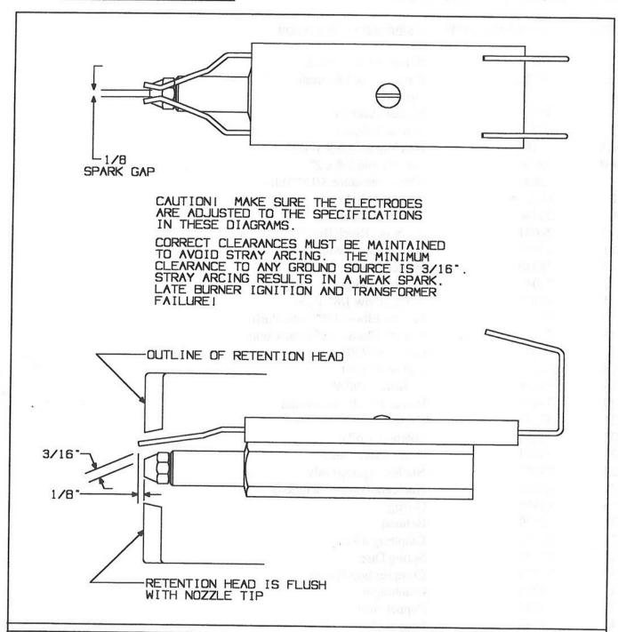
The burner electrodes should be replaced annually to maintain proper burner performance.
